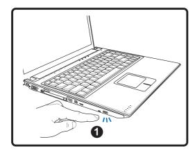
1. While the Notebook PC's power is ON, press the drive's eject button and the tray will eject out partially.
